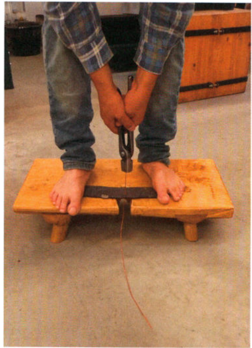
Abb. 4: Gezogener Kupferdraht (rund) am Ziehschemel. – Drawn copper wire (round diameter) at the foot stol.
